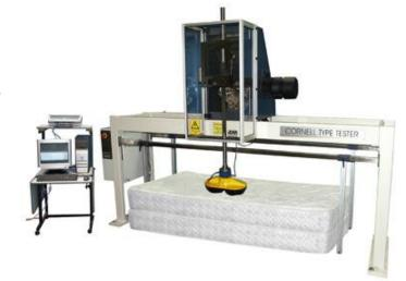
The bedding is located below the ram, and the eccentric and shaft position adjusted so that the maximum load of 1025N and the minimum load of 22N is applied when the eccentric is rotated to the lowest and highest positions respectively. A position transducer is located so the position of the ram head can be measured automatically.
